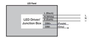
To wire multiple dimming panels to one standard 0-10v dimmer use the schematic below. The maximum number of panels that can be dimmed depends on the capability and capacity of the dimmer. Wire using plenum rated low voltage wire and appropriate connector.
