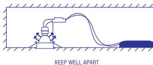
(Figure.2 - INCORRECT Installation)
